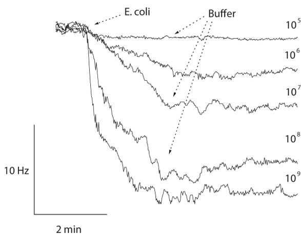
**Figure 2.** The acquired response curves (resonant frequency vs. time), recorded for samples containing different *E. coli* levels, measured by the piezoelectric immunosensor with immobilized polyclonal antibody specific against *E. coli*. The arrows indicate addition of the *E. coli* sample and/or carrier buffer flow.
