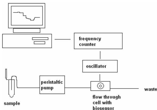
**Figure 1.** Block diagram of the piezoelectric immunosensor system. The signal collecting part is expressed by PC, frequency counter, and oscillator connected with the sensor. The flow through part consists of the microtube with sample, peristaltic pump, and flow through cell containing the sensor sandwiched between two soft o-rings. Only one side of the piezoelectric sensor is contacting the solution.
