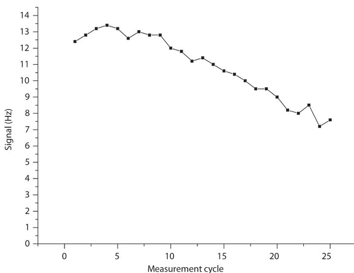
**Figure 4.** Long term stability of the immunosensor. Responses from the sequence of measurements of the same sample *E. coli* at  $10^8$  CFU/mL.
