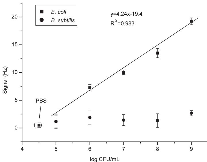
**Figure 3.** The calibration plot (signal in Hz vs. log of cell content) represents dependences obtained with *E. coli* (■) and negative control *B. subtilis* (●), respectively. The point in brackets represents the background signal obtained with PBS. The error bars represent estimated standard deviations ( $n = 3$ ).
